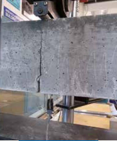
CMOD controlled bending test in compliance with EN 14651 standards
