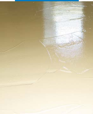
The fresh surface of Mapecolor Paste after application with a trowel
